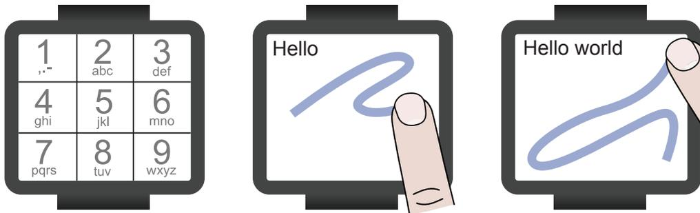
**Figure 1:** Invisiboard combines T9 text entry with swiping, to enable fast text entry on tiny screens while maximizing display space. Left: The screen is divided into nine areas, each containing 3-4 characters. Middle, Right: During use, the keyboard remains invisible. The user swipes across the desired keys and the software presents words based on a language model. If necessary, the user can scroll through available words, ordered by probability.
