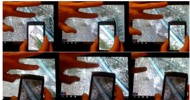
Figure 4 – Top: The phone is touching the tablet. Because the two are coupled the pan gesture is executed on both devices. Bottom: The phone is no longer touching the tablet. The pan gesture is executed on the tablet, while the phone remains static.
